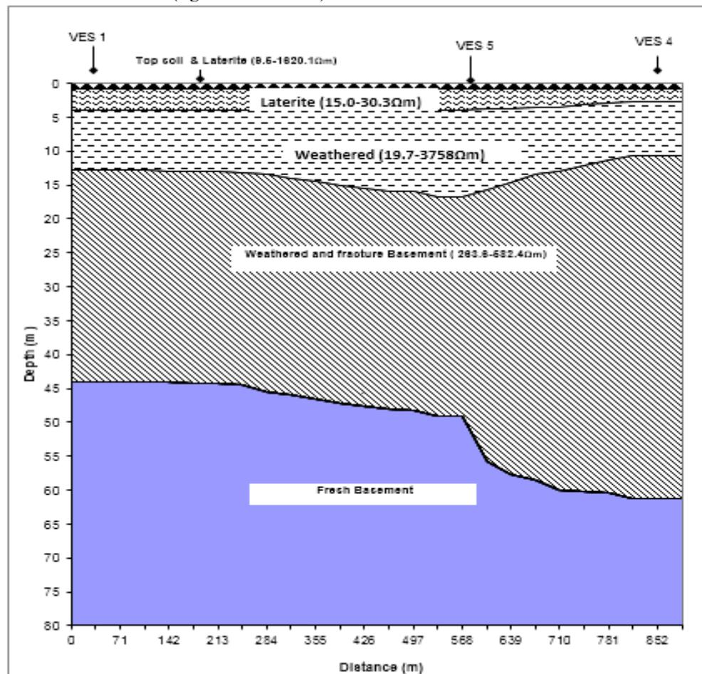
Fig 10: Geoelectric section of VES (1, 4, 5)
