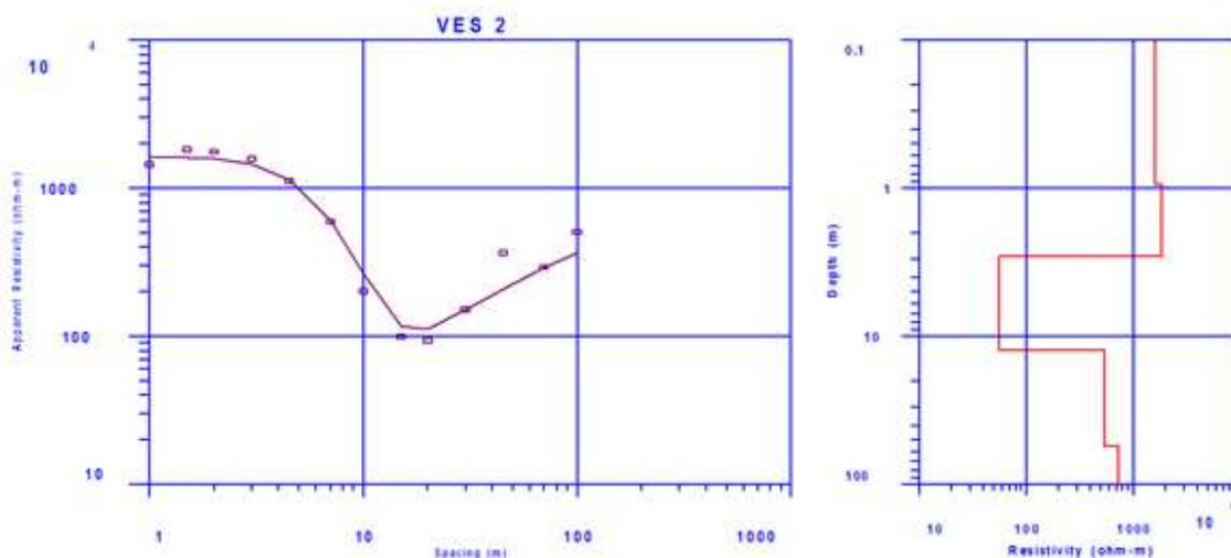
Figure 4: Resistivity curve for VES 2.
