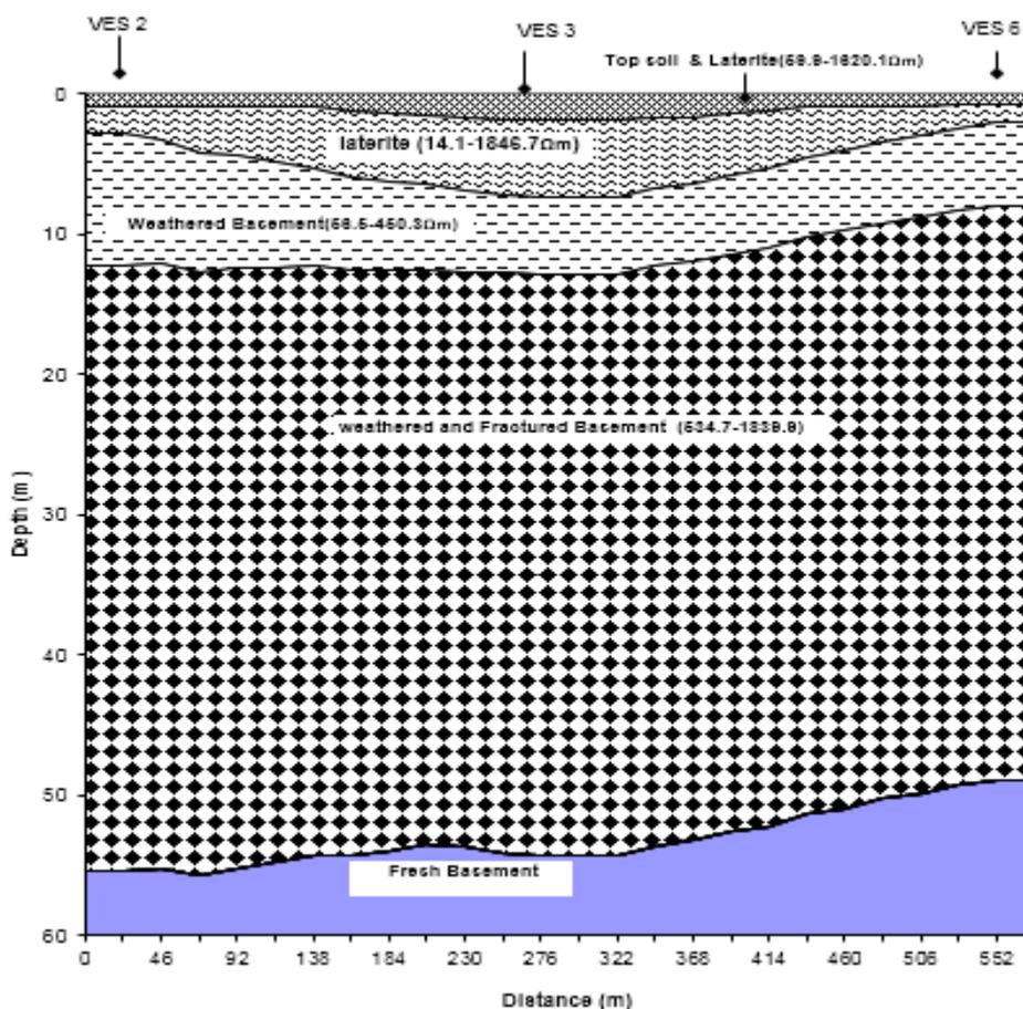
Fig 11: Geoelectric section of VES (2, 3, 6)
